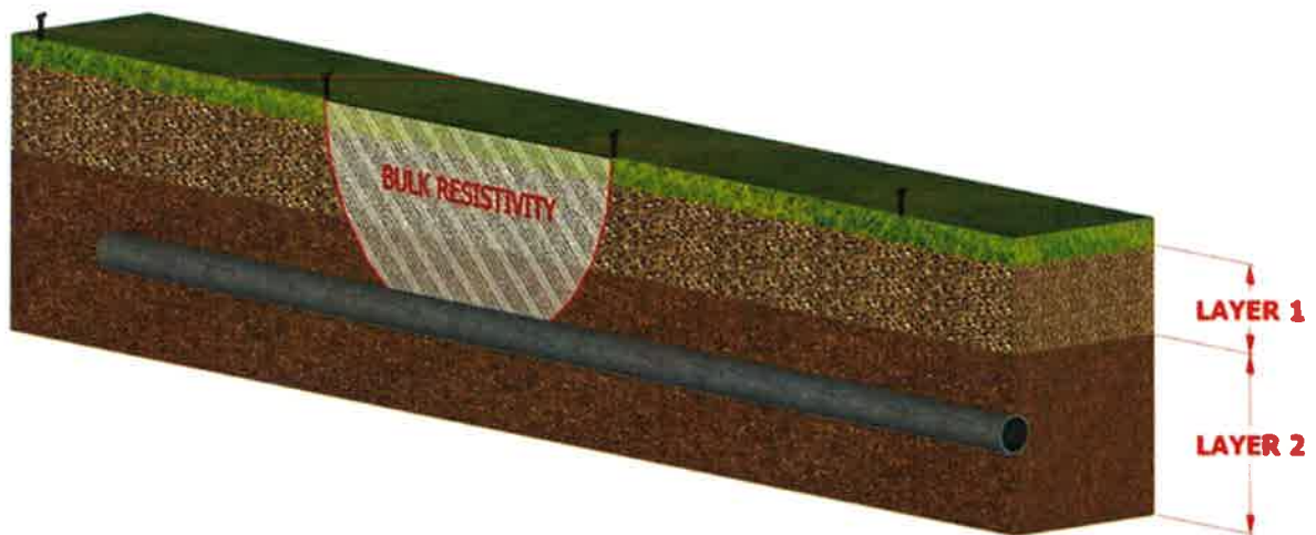
Figure 9. Graphical representation of soil resistivity measurements, showing bulk and layer zones
