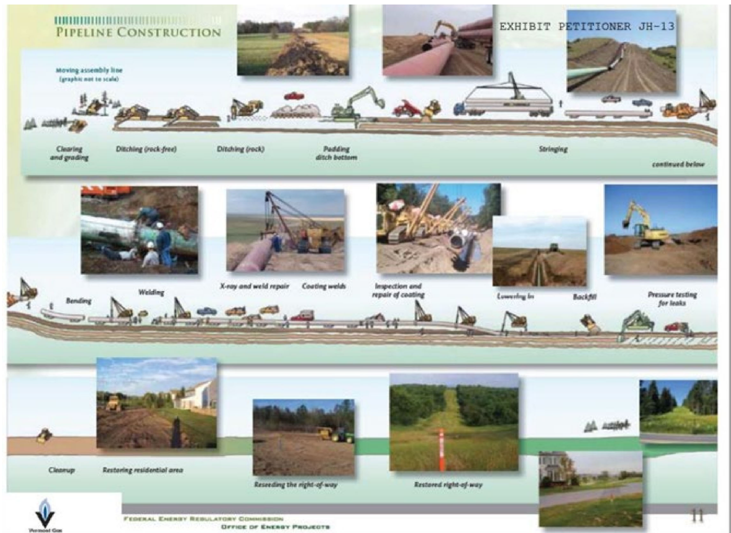
Figure 1. Pipeline Construction Diagram
