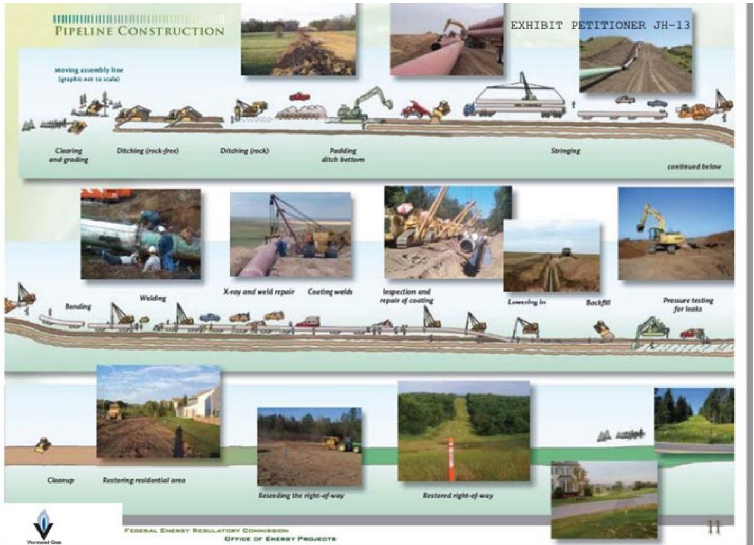
Figure 1. Pipeline Construction Diagram
